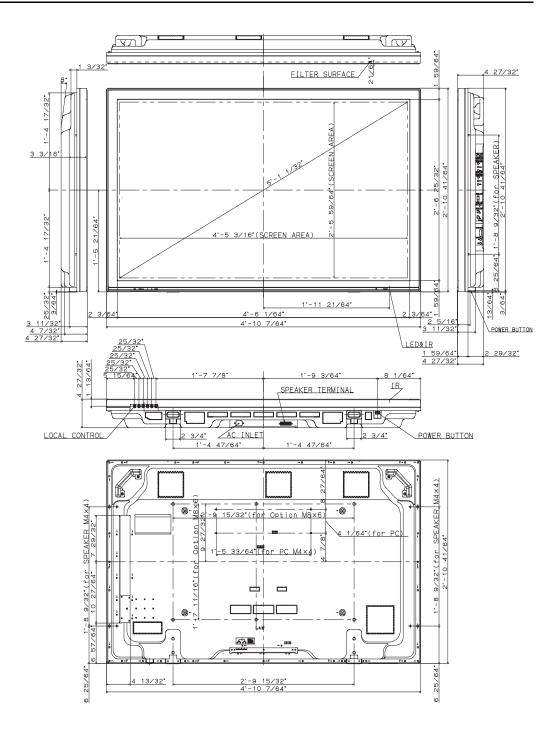
Figure 7-2. PlasmaWall Model PL-61DHD Dimensions
